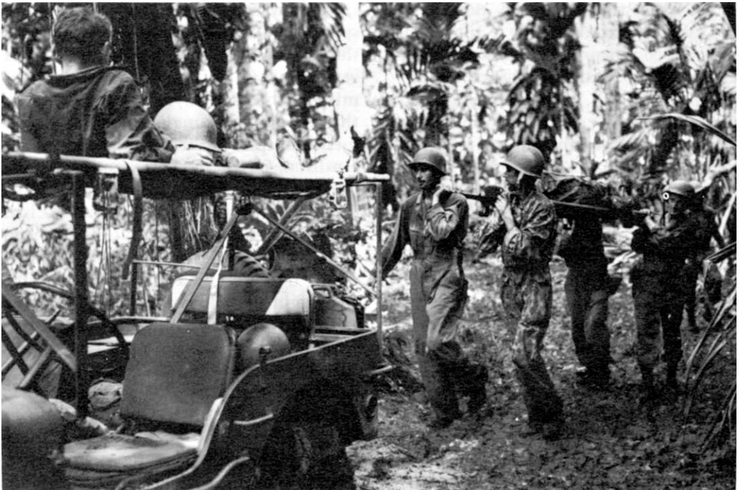
EVACUATING CASUALTIES, 12 JULY 1943. Jeep, converted into an ambulance, could carry three litters and one sitting patient.
